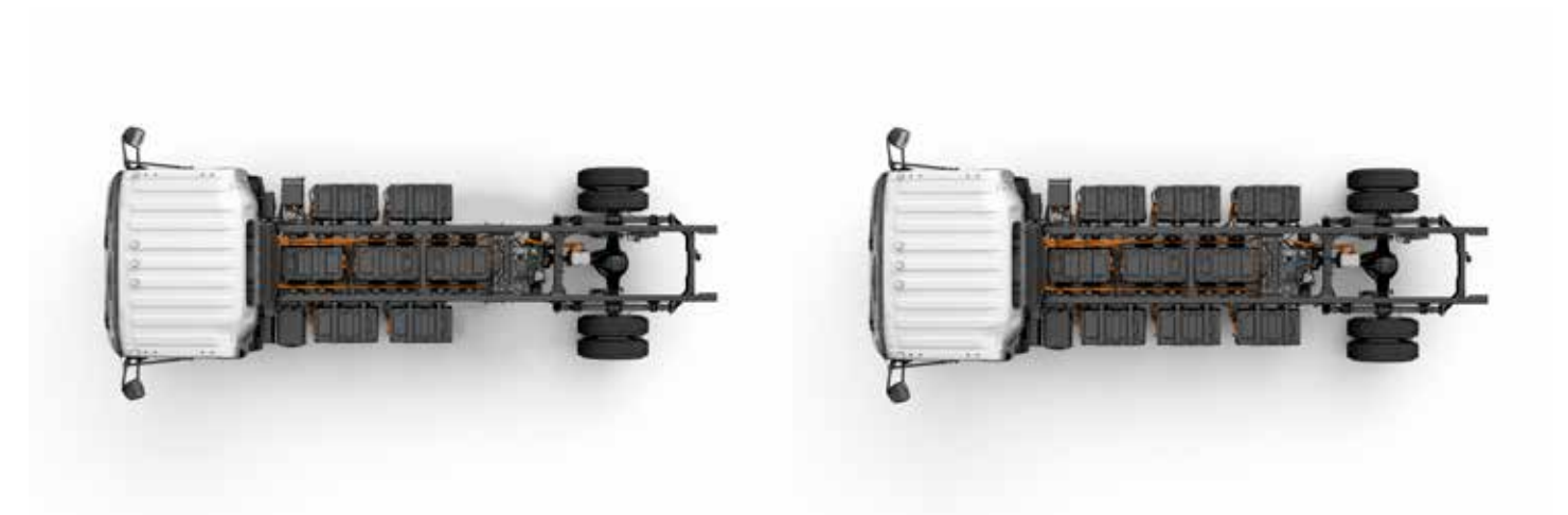
7 Battery Packs - 140 kWh
